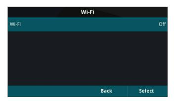
To enable this functionality, navigate down to "On" and press the "Select" key.
